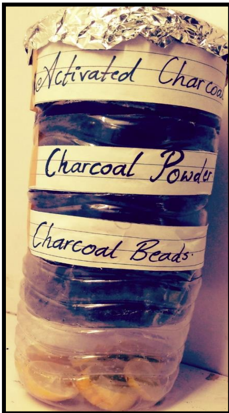
Fig. 3 Combination filter of charcoal with lemon slices
