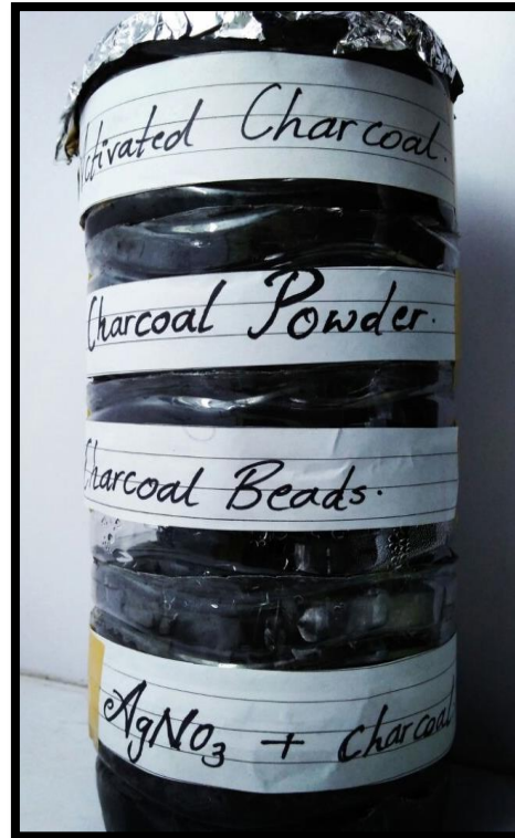
Fig. 2 Combination filter of charcoal with heavy metal
